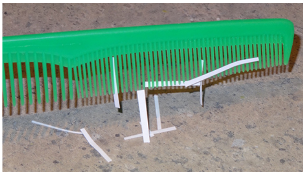
Figure 5.3 After being used to comb hair, this comb attracts small strips of paper from a distance, without physical contact. Investigation of this behavior helped lead to the concept of the electric force. (credit: Jane Whitney)
