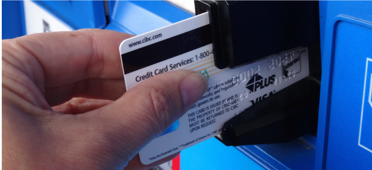
Figure 13.1 The black strip found on the back of credit cards and driver's licenses is a very thin layer of magnetic material with information stored on it. Reading and writing the information on the credit card is done with a swiping motion. The physical reason why this is necessary is called electromagnetic induction and is discussed in this chapter. (credit: modification of work by Jane Whitney)
