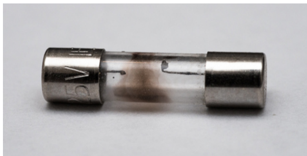
Figure 9.25 A fuse consists of a piece of wire between two contacts. When a current passes through the wire that is greater than the rated current, the wire melts, breaking the connection. Pictured is a “blown” fuse where the wire broke protecting a circuit (credit: modification of work by “Shardayyy”/Flickr).
