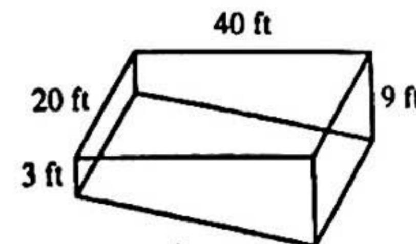
$$(b) F = \int_0^9 \delta x 20 dx = 20\delta \left[ \frac{1}{2}x^2 \right]_0^9 = 20\delta \cdot \frac{81}{2} = 810\delta = 810(62.5) = 50,625 \text{ lb} \approx 5.06 \times 10^4 \text{ lb.}$$
