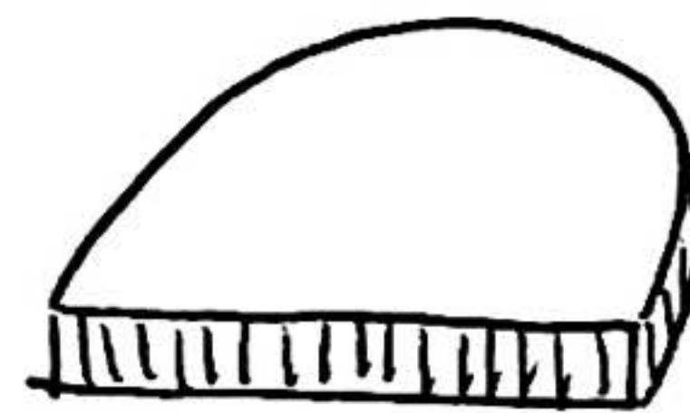
$$\begin{aligned} dV &= A dy \\ &= \frac{1}{2}\pi x^2 dy \\ &= \frac{1}{2}\pi 25y dy \end{aligned}$$
