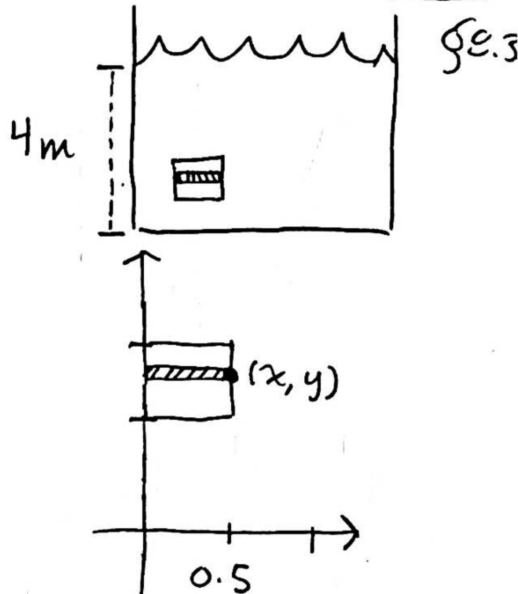
A DIVING POOL THAT IS 4m DEEP & FULL OF WATER HAS A VIEWING WINDOW ON ONE OF IT'S WALLS. FIND THE FORCE ON A WINDOW THAT IS SQUARE,  $\frac{1}{2}$ m on a SIDE, w/ THE LOWER EDGE OF THE WINDOW 1M FROM THE BOTTOM OF THE POOL.
