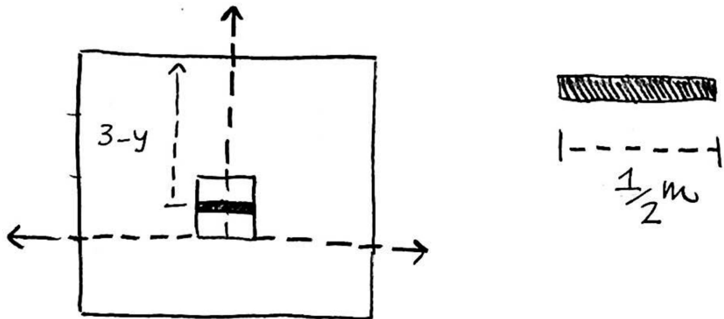
$$\begin{aligned} F &= PA \\ &= \rho gh (\frac{1}{2}) \Delta y \\ dF &= 9800 (3-y) \frac{1}{2} dy \end{aligned}$$
