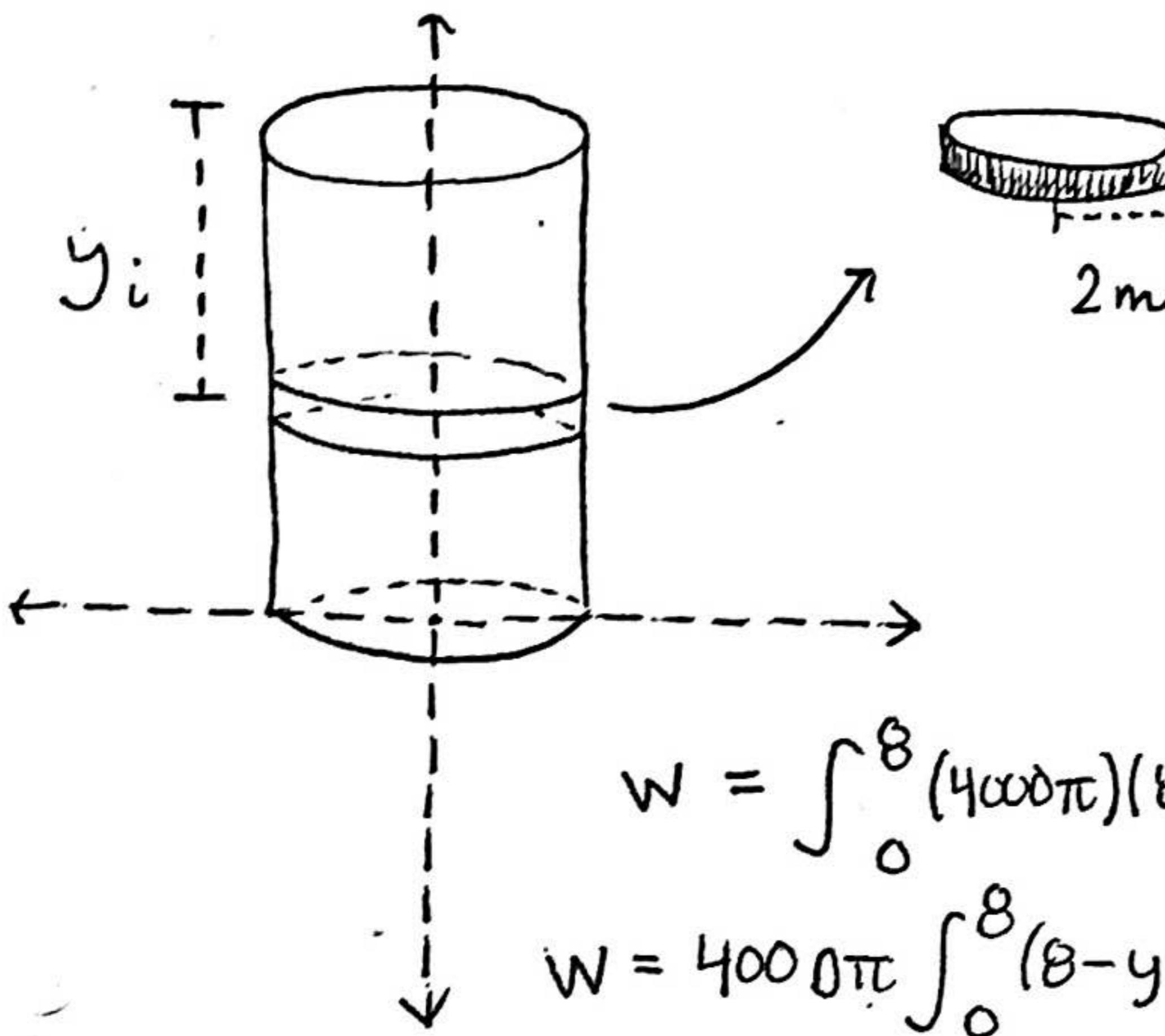
$$\begin{aligned} W_i &= F \cdot d_i \\ &= \rho V_i \cdot d_i \\ &= \frac{1000 \text{ kg}}{\text{m}^3} \pi r^2 \int A y \\ &= (1000) \pi (2)^2 \int \Delta y \\ &= 4000\pi (8 - y_i) \Delta y \end{aligned}$$
